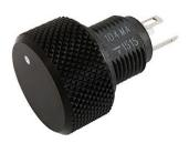
The P16 is a revolutionary concept in panel mounted potentiometers. This unique design consists of a knob driving and incorporating a cermet potentiometer. Only the mounting hardware and terminals are situated on the back side of the panel reducing to a minimum the required clearance.
